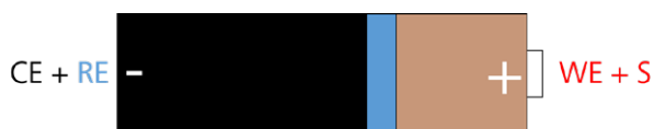
Figure 4. A battery with two electrodes. The negative electrode hosts the counter and reference leads, while the positive electrode hosts the working and sense lead.
